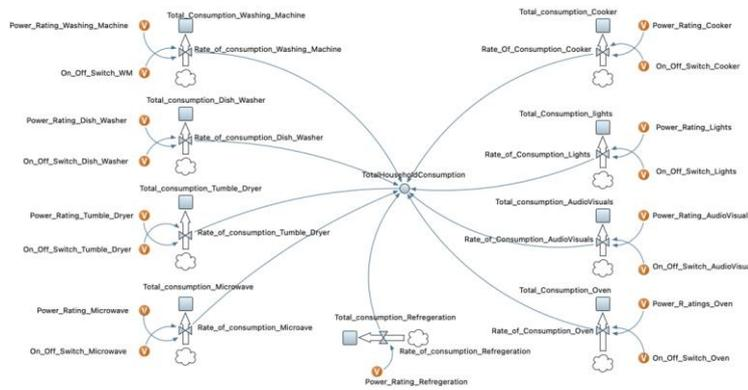
Fig. 2. Anylogic model of the nine HH appliances.
