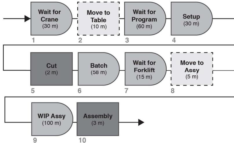
**Fig. 4.** – Product Path Diagram (Fabrication)
