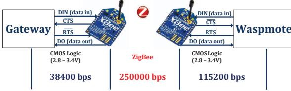
Fig. 3. Serial and wireless communications between XBee-based devices
