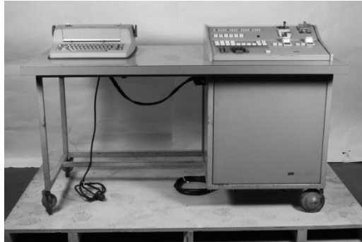
Figure 10: Pacific Data Systems PDS 1020 mini desktop computer. Desktop with typewriter and paper tape input/output Photo courtesy of Museum Victoria
