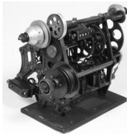
Figure 4: Electro-mechanical Totalisator: ‘Julius Horse Adder’, c 1926
