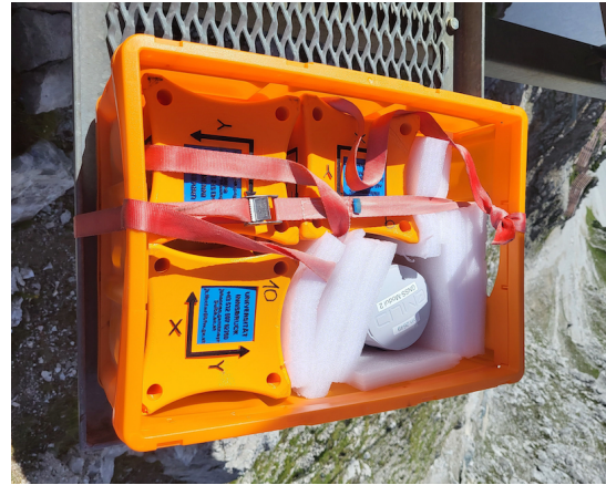
Figure 10. Equipment box fastened onto the cable car counterweight. The box contained both an AvaNode as well as a high precision GNSS system.
