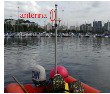
Fig. 4. Gateway installed on the coach's boat
