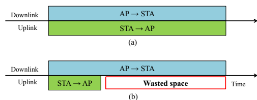
Fig. 1. Uplink and downlink frame size comparison. (a) Ideal full-duplex frame size. (b) Full-duplex frame size in real-world traffic.
