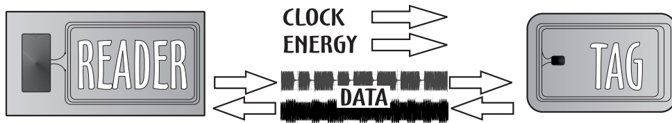
Fig. 1. RFID Operation Principle.
