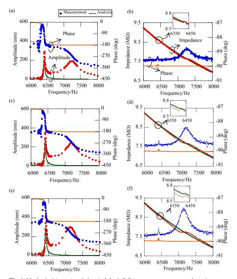
**Fig. 6.** Mechanical (a, c, e) and electrical (b, d, f) frequency responses around x-axis resonance mode at bias voltage (a, b) 5 V, (c, d) 6 V, (e, f) 7 V.
