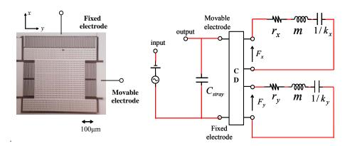
Fig. 5. In-plane 2DOF SOI resonator
