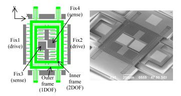
Fig. 8. In-plane decoupled 2DOF resonator (a) schematics and (b) fabricated device for SOG gyroscope
