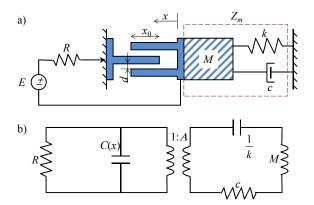
Fig. 1. Simple equivalent circuit model of one-degree-of-freedom comb resonator.
