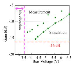
**Fig. 14.** Simulated and measured total gain of the electrostatic resonator and transimpedance amplifier as a function of bias voltage.
