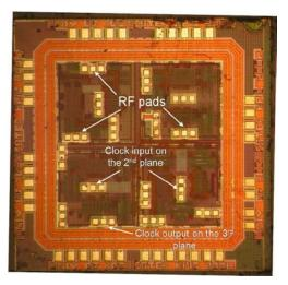
Fig. 9. Fabricated 3-D test circuit. The total area is 3 mm  $\times$  3 mm. There are four different blocks, with one input and three output RF pads for each block. The area of each block is approximately 1 mm<sup>2</sup>.
