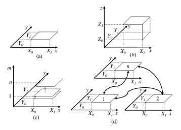
**Fig. 4.** Example of physical design solution space for floorplanning 2-D and 3-D circuits, (a) available area for floorplanning a planar circuit, (b) available volume for floorplanning a 3-D circuit, (c) a finite number of planes is considered to reduce the solution space, and (d) the floorplan of the planes is generated after the circuit cells are assigned to each plane. The arrows represent global constraints among planes that guide the floorplan of a 3-D system.
