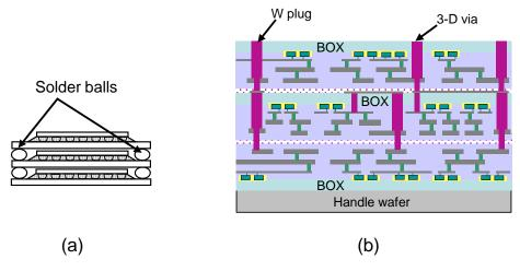
Fig. 2. Different forms of 3-D integration (not to scale), (a) system-in-package (SiP) [17] and (b) a 3-D circuit with dense through silicon vias [20], [21]. Two different bonding styles, frontto-front and front-to-back, are illustrated. The W plug is composed of tungsten.
