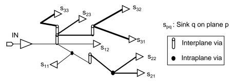
Fig. 8. An example of an interplane interconnect tree.
