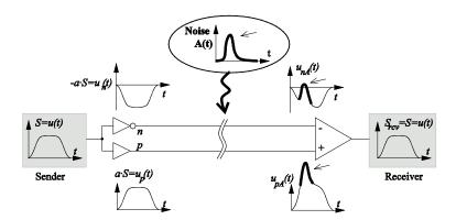
Fig. 4. Functional principle of a differential pair.
