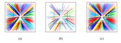
**Fig. 12.** Pin assignment for a single chip module using defensive blending. (a) Fat pin assignment. (b) Assignment of remaining pins and nets. (c) The final pin assignment with 454 possible differential pairs is the combination of (a) and (b).
