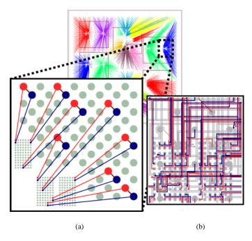
**Fig. 16.** Details of a differential pair pin assignment. As illustrated by the shown subset of flylines in (a), each differential pair is assigned adjoining chip and MCM pins (smaller and larger dots) with distances of less than  $d_{max}$ . The final routing result of differential pairs is shown in (b). Note that (a) contains only a small subset of differential pairs, non-differential pairs are omitted for simplicity.
