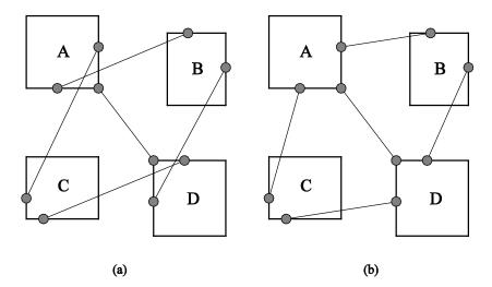
**Fig. 2.** Example with four components A-D to illustrate the influence of pin assignment on the routability. Pins are marked by circles ● on the outline of the components. Nets are shown as flylines. If no wiring is allowed below components A through D, the design with pin assignment (a) is not routable in one layer, whereas (b) allows single layer routing.
