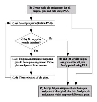
**Fig. 14.** Major steps of pin assignment with differential pairs using defensive blending. This figure extends Fig. 7 in which the interaction of the basic pin assignment and the process of selecting pin pairs is indicated as a dashed arrow from step 4 to step 1.
