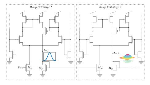
Fig. 6. By connecting the diode-connected output transistor to the tail transistor of the next stage bump cell, the resulting output current can approximate a multivariate Gaussian function with a diagonal covariance matrix.
