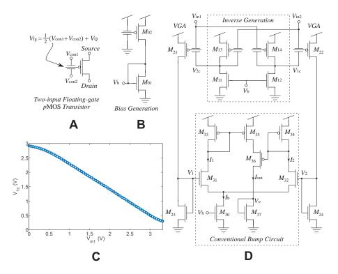
Fig. 3. A: The symbol of a two-input floating-gate pMOS transistor. B: The schematic of the bias generation circuit for the proposed floating-gate bump circuit. C: The transfer characteristic of the inverse generation block. D: The schematic of the proposed bump circuit that is composed of an inverse generation block, a fully differential variable gain amplifier (VGA), and a conventional bump circuit.
