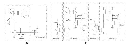
**Fig. 9.** A: The schematic of the "FG-pFET & Mirror" block. The charge on the pMOS transistor can be programmed to set the height of the bell-shaped transfer curve. B: The schematic of a current mode winner-take-all circuit. Only the output voltage of the winning cell will be high to indicate the best-matching template.
