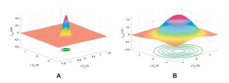
Fig. 7. Measurement results from two cascading floating-gate bump circuits.  $\Delta V_{\rm X}$  is the input voltage difference  $\Delta V_{\rm in} = V_{\rm in1} - V_{\rm in2}$  of the first stage floating-gate bump circuit and  $\Delta V_{\rm Y}$  is the input voltage difference of the second stage. In both stages,  $V_{\rm in2} = V_{\rm DD}/2$ . The common-mode charges are programmed to different levels to approximate bivariate Gaussian functions with different variance.
