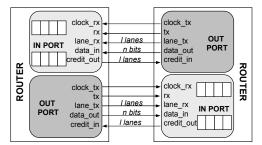
Fig. 1. Physical router interface for the BE-NoC.
