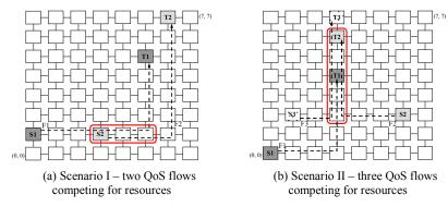
**Fig. 5.** Spatial traffic distribution of source and target nodes for flows with QoS requirements. Dotted lines indicate the path of each flow. Rounded rectangles highlight the area where flows compete for network resources. All other nodes transmit *C* flows, disturbing the QoS flows.
