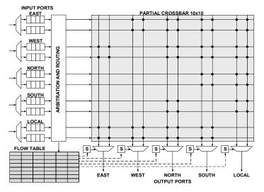
Fig. 3. Router architecture with support for rate-based scheduling.
