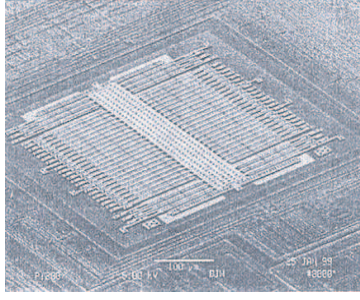
Fig. 5. Die photo of ADXL103 sensor region (4x3 self-test cells and 42 sense cells). (Source: Analog Devices; reprinted with permission.)
