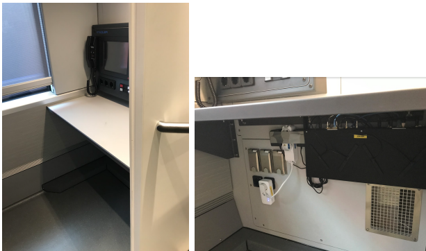
(a) Conductor cab (b) Node under desk Fig. 1: Node deployment on trains in Norway.
