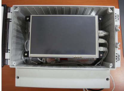
Fig. 8. Embedded board including environment sensor receiver, database, and the web server
