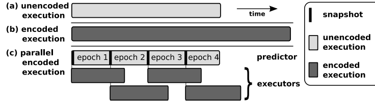
Fig. 3. (a) Original application execution without encoding and parallelization. (b) Sequential execution with encoding. (c) Parallelized encoded execution. Unencoded predictor for fast state prediction. Parallelized executors execute slow encoded variant.
