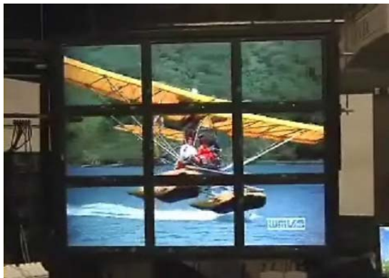
Fig. 4. Snapshot of Tiled Display on LCD Array
