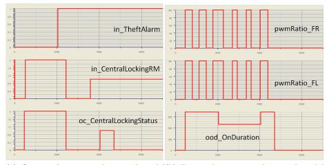
(a) Generated inputs and internal model(b) Expected outputs and internal model state oc\_CentralLockingStatus. state ooo\_OnDuration.
