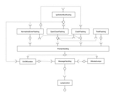
Fig. 2: First-level decomposition of system under test.
