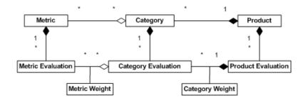
*Figure 1.* An UML diagram illustrating the evaluation meta-model, where a single metric can influence more than one category, and weights are used to take into account the final rating's dependency from the evaluation context.
