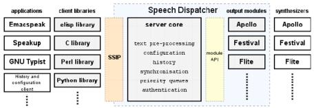
Fig. 2. Speech Dispatcher architecture and interfacing
