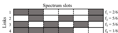
Fig. 1. An example of spectrum slot occupancy states of various optical links. The shaded areas are the occupied slots.
