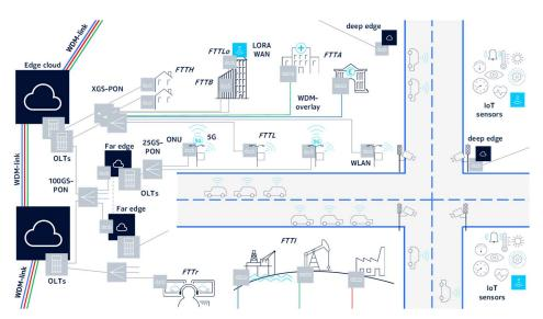
Fig. 1. Smart city infrastructure using PON as the backbone. PON provides connectivity to the households and antenna sites, and is used as a low-cost aggregation system to transport the data from far edge clouds to the main edge clouds.
