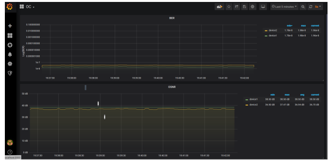
Fig. 2. Parallel telemetry of Multi-Xponder OSNR and BER collectors with Grafana-based GUI [15]
