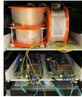
Fig 3. Photograph of the two FPGAs with our real-time implementation separated by 10km single mode fiber
