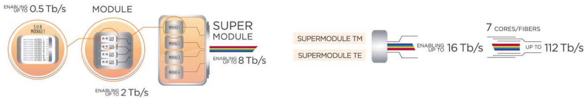
Fig. 3. Multi-Tb/s S-BVT transmitter based on VCSEL integration with modular approach.
