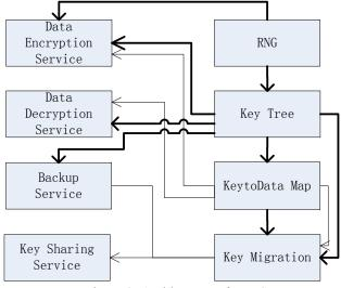
Figure 2: Architecture of PDPS
