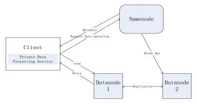
Figure 6: Architecture of HDFS with PDPS
