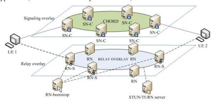
Fig.1 P2P VoIP system structure
