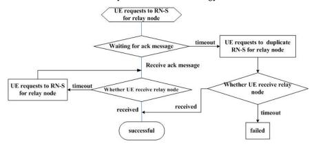
Fig. 5 Redundancy detecting
