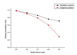
Fig. 9 Dialog completion ratio with node failure ratio
