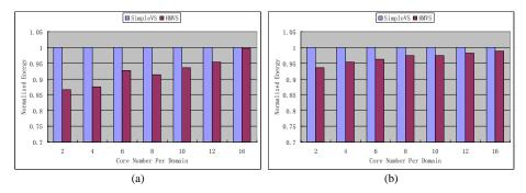
**Fig. 4.** Normalized energy consumption under different VFD granularity (a) The average core utilization  $acu \in [0.3, 0.4]$ . (b) The average core utilization  $acu \in [0.6, 0.7]$ .
