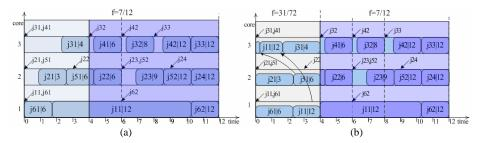
**Fig. 2.** (a) Adjust the slack times by shifting them forward. (b) Reallocate the slack times and scale down the operation frequency in [0, 4].
