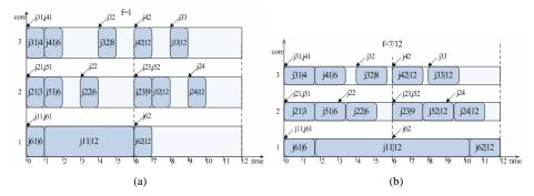
**Fig. 1.** (a) Schedule the tasks by EDF algorithm without the voltage scaling. (b) Schedule the tasks with the static SimpleVS algorithm.
