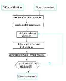
Fig. 6. Flow of Pemvin simulation
