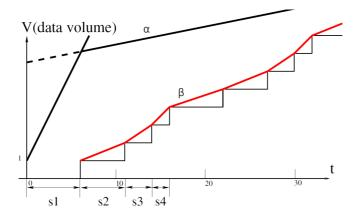
**Fig. 5.** Service curve of TDM VC ( $s_i$  stands for a session)  $\alpha$  is the arrive curve and  $\beta$  is the service curve.
