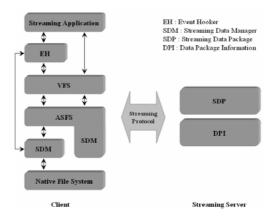
Fig. 1. Architecture of client and streaming server in the ASOD system
