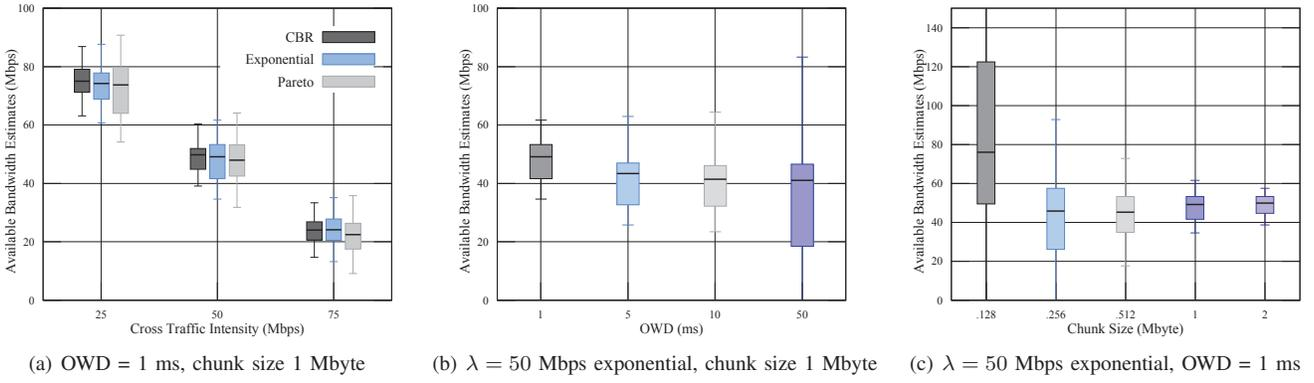
Fig. 7. Parameter evaluation. Bandwidth estimates for different types of cross traffic burstiness (a), OWDs (b), and chunk sizes (c). The quality of the estimates is good for small to medium OWDs and improves with the chunk size. The burstiness of cross traffic mostly influences the variability of the estimates.
