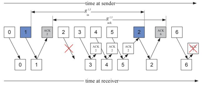
Fig. 10. Use of the ack-gap model in the presence of packet loss. Duplicate acknowledgements are ignored and the ack-gap is closed by the next higher cumulative acknowledgement. The corresponding input gap has to consider the retransmission that triggered this acknowledgement.
