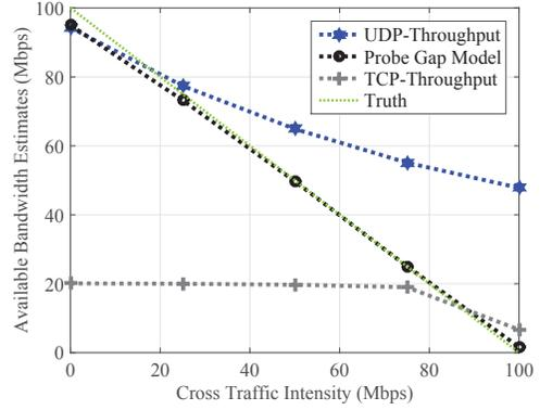
Fig. 5. Available bandwidth estimates for varying cross traffic rates. The estimates obtained from UDP  $(g_{in}, g_{out})$  measurements closely match the ground truth. The TCP throughput underestimates the available bandwidth, mainly due to the OWD of 10 ms and the limited chunk size of 1 Mbyte. The UDP throughput overestimates the available bandwidth since a greedy UDP sender can preempt cross traffic at a FIFO multiplexer.
