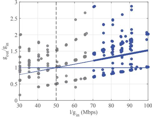
Fig. 4.  $(g_{in}, g_{out})$  samples obtained by transmission of a chunk of 1 Mbyte via UDP. The sender varies  $g_{in}$  so that the samples are evenly distributed. Samples that are marked blue are used to determine the regression line. The intersection of the regression line with the horizontal line at 1 marks the available bandwidth of 50 Mbps.
