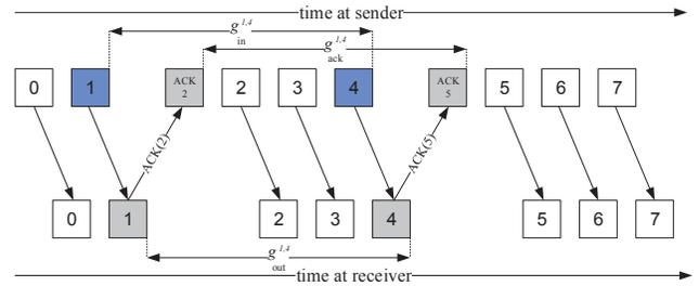
Fig. 8. Multi-gap and ack-gap models. The ack-gap enables available bandwidth estimation using sender-side measurements only.
