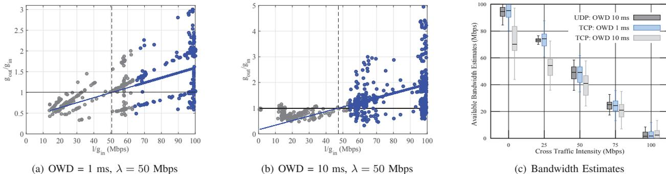
Fig. 6.  $(g_{in}, g_{out})$  samples obtained from passive TCP measurements and bandwidth estimates obtained thereof. The values of  $g_{in}$  are a result of TCP congestion control and depend on network parameters such as the OWD. With increasing OWD a clustering of  $g_{in}$  samples is observed and the variability of bandwidth estimates increases.
