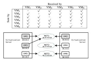
Fig. 5: Virtual network topologies used to evaluate MAC address resolution. All logical networks were implemented over the physical network in Fig. 3.
