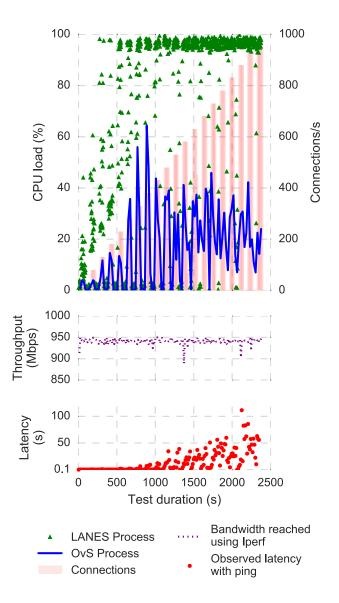
Fig. 10: Load test results for LANES.
