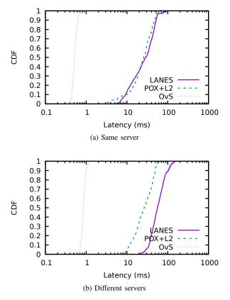
Fig. 8: Latency for installing OpenFlow rules on switches
