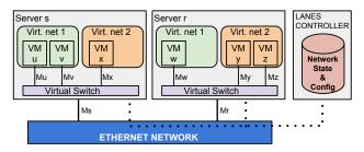
Fig. 1: LANES perspective of an example deployment in a multi-tenant datacenter.
