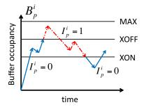
Fig. 3. Buffer occupancy over time for ingress queue buffers.
