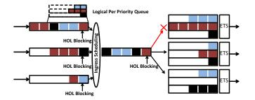
Fig. 1. The switch architecture and the HOL blocking
