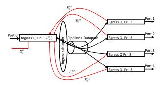
Fig. 5. Packets from a single ingress queue are forwarded to all egress queues per-priority. In return, the ingress queue receives a congestion state signal from each egress queue per-priority.
