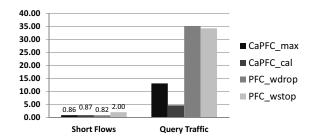
Fig. 9. Tail FCT (ms) results for all techniques in a shared memory switch.  $V. \quad RELATED \ WORK$
