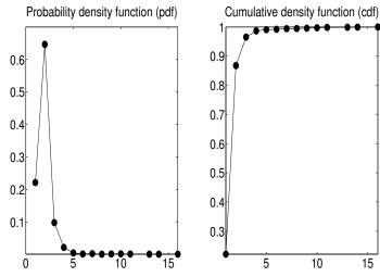
Fig. 2: Aggregated degree distribution of sub-stations in the dataset showing majority of sub-stations have low connectivity.
