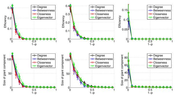
Fig. 5: (Color Online) The impact of cascading failures on the communication efficiency,  $\eta$  (top row) and the size of giant component (bottom row) when 1-p fraction of nodes are removed based on different targeted attacks for an MV grid coupled with N>30 interdependent on ER (left column), SW (center column) and SF (right column) graph.
