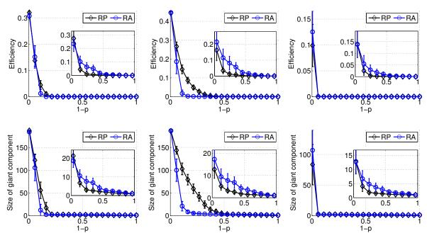
Fig. 4: (Color Online) The impact of random cascading failures on the communication efficiency (top row) and the size of giant component for an MV grid (bottom row) when 1-p fraction of nodes are removed based on RP and RA strategies for an MV grid with N > 30 (Inset: grid with N < 30) coupled with ER (left column), SW (center column) and SF (right column) graph.
