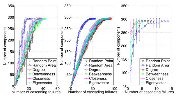
Fig. 6: (Color Online) Effect of cascading failures on the number of resulting components for MV grid coupled with ER (left), SW (center) and SF (right) networks.
