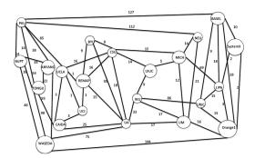
Fig. 7. A replica of the actual NDN testbed topology which contains 22 nodes and 50 links.
