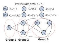
Fig. 8. Example of packet grouping.
