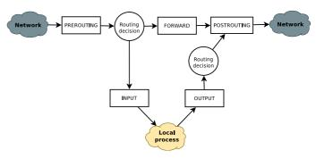
Fig. 2: Linux routing mechanism
