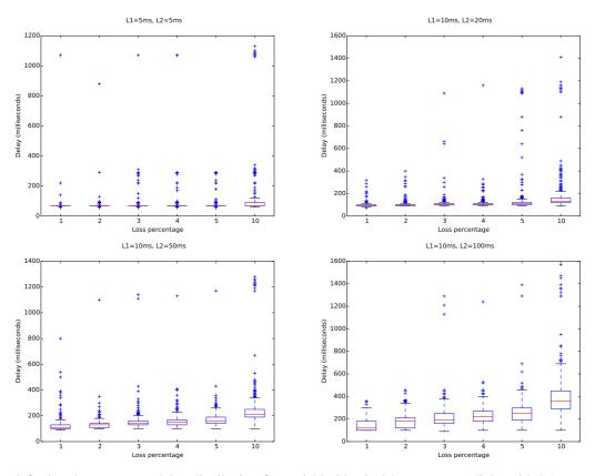
Fig. 5: Upper left plot shows request delay distribution for variable identical loss over two links with L1 set at 5ms delay and L2 set at 5ms. Upper right plot shows the same for L1 at 10ms and L2 at 20ms. Bottom left plot shows for L1 at 10ms and L2 at 50ms. Bottom right plot shows for L1 at 10ms and L2 at 100ms.
