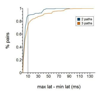
Fig. 9: For P = 2, 3 and  $\Delta d$  we show the percentage of pairs that have a difference of latency between the IGP path and the worst path in the path set found by our algorithm at most  $\Delta d$ .
