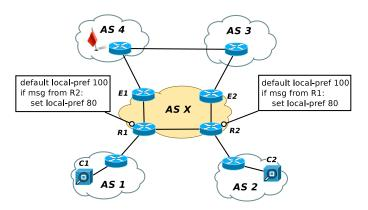
Fig. 1. Example BGP network with two vantage points (i.e., C1 and C2) and an AS deploying iBGP policies (i.e., AS X).
