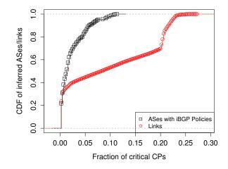
Fig. 5. Comparison of the fraction of critical CPs for topology discovery (circles) and iBGP policy inference (squares).
