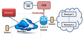
Fig. 1. SIP Misuse Detection Network Architecture
