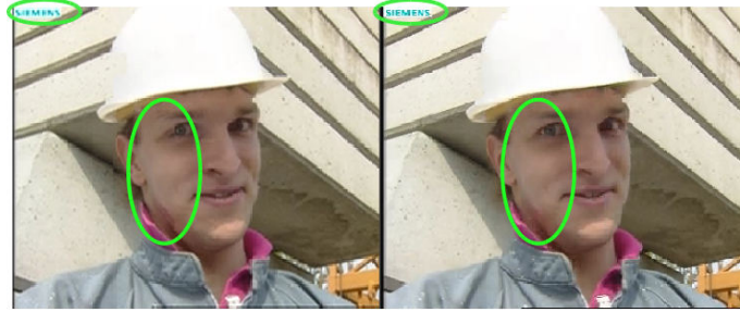
Fig. 8: Effect on the perceptual video quality of the base layer (Left: Opportunistic CA 288x216 - 579 kbps, Right: Proposed CA 352x288 - 703 kbps)
