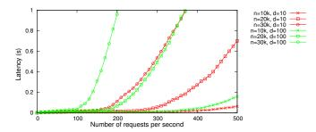
Fig. 12. Matching time measurement: plain-text(red) vs. encrypted message(green)
