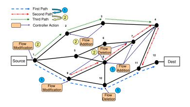
Fig. 10. Controller involvement in re-routing flows
