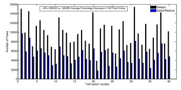
Fig. 7. Compression achieved by SwitchReduce on ToR switches
