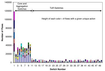
Fig. 4. Action overlap on Host ToRs and Aggregation/Core switches
