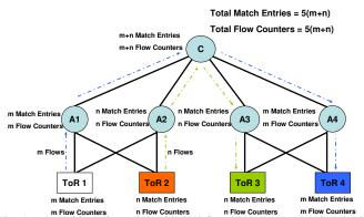
Fig. 1. Repetition of match entries and flow counters at every hop in the network
