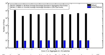
Fig. 6. Compression achieved by SwitchReduce on Aggregation/Core switches
