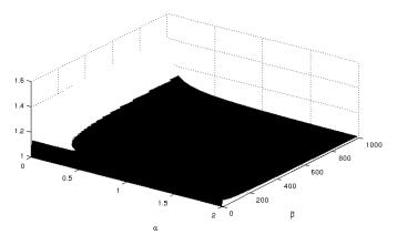
Fig. 4. Evolution of the *inefficiency* as a function of  $\alpha$  and  $\beta$  for K = 5 dispatchers.
