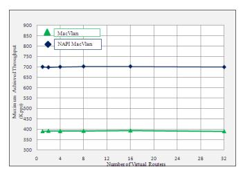
Fig. 6. Throughput vs. no. of virtual routers
