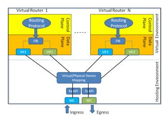
Fig. 1. General design of Linux-based virtual routers
