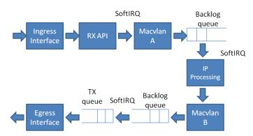
Fig. 2. Data plane for a macvlan based virtual router
