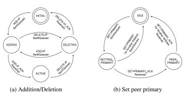
Fig. 3. State transition diagram for local addresses.
