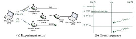
**Fig. 2.** Problem 2 – The ADD-IP operation cannot be generated after IP1 is up at time t3 because IP1 is still in the association (under deletion). (Acronyms in the figure: IP – IP Address; IF – Interface; WR – Wireless Router)
