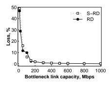
Fig. 3. Capacity scalability of the S-RD algorithm: (a) maximum queuing delay of class D; (b) comparison of the loss rate for class D to original version of the RD link.
