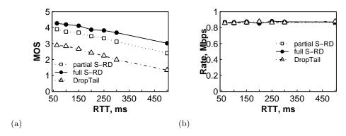
**Fig. 5.** Performance under the partial deployment for different propagation RTTs: (a) Average MOS; (b) average per-flow throughput of class R.
