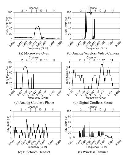
Fig. 4. Duty cycle analysis for six non-Wi-Fi devices
