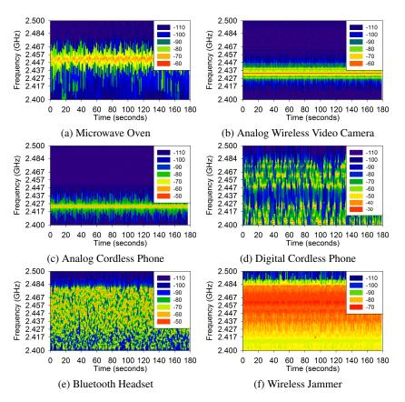
Fig. 3. Spectrograms for six non-Wi-Fi devices
