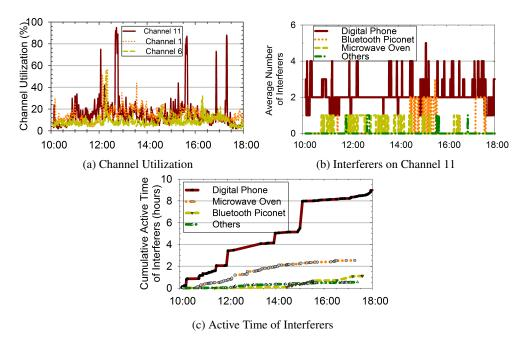
Fig. 6. Passive measurements from campus Wi-Fi network
