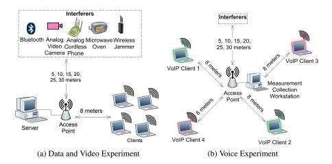
Fig. 1. Experimental setup
