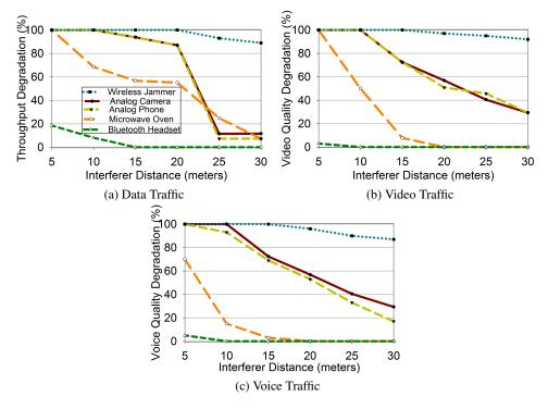
Fig. 5. Impact of interference on different workloads
