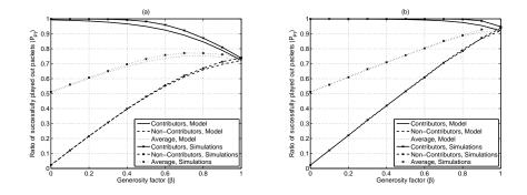
Fig. 1. Ratio of successfully played out packets vs generosity factor  $\beta$  for playback delay of (a) B = 10 and (b) B = 40. Analytical and simulation results.
