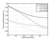
Fig. 2. Ratio of duplicate transmissions vs generosity factor ( $\beta$ ) for B = 10 and B = 40. Simulations.
