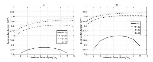
Fig. 4. Social welfare versus reserved server capacity for different playback delays. Linear (a) and logarithmic (b) utility functions. Overlay with N = 500, d = 30 and m = 11.
