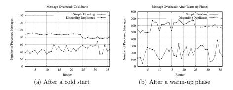
Fig. 5. Message overhead of all mesh routers
