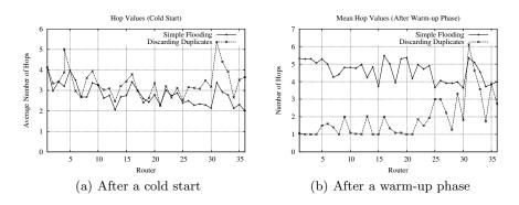
Fig. 6. Mean hop count values of received messages of all mesh routers
