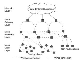
Fig. 1. Wireless Mesh Network architecture
